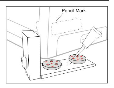
5. Quickly and carefully place the PTL in the marked area on the printer and apply **firm** and **steady** pressure for 100 seconds.
