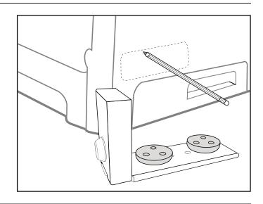
3. Use the provided alcohol wipes to **thoroughly** clean inside the marked area on the printer as well as the flex feet. (Clean entire surface of rubber on PTL-3R/5R.)
