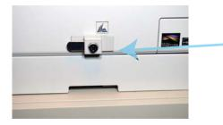
The Mini is left in the "unlocked" position while drying
