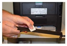
3. Apply the adhesive down the middle of the base plate. Press the base plate firmly onto the marked area and hold for 2 minutes. Try to work out any air pockets and wipe away excess glue.
